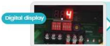
Digital display on the PCB, it can show system's operation status and error codes.
